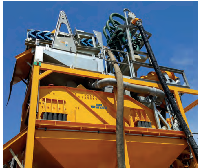
Grobsieb und Desilter (optional) Coarse screen and desilter as options
